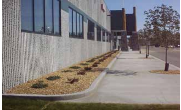
Example of completed front landscape planters complete with landscape fabric, mulch/stone, plantings with soaker/drip type irrigation.
